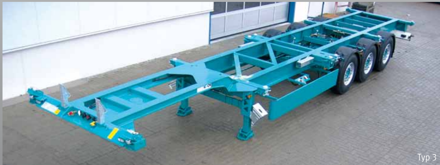
Containerchassis Typ CCS/GF Hafenchassis
